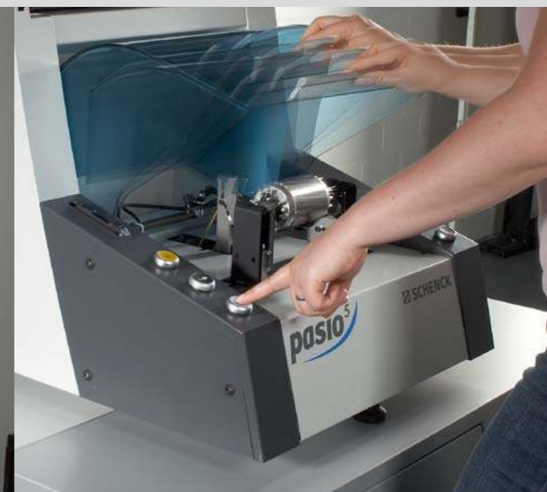
Protective cover for rotors with sharp-edged surfaces
