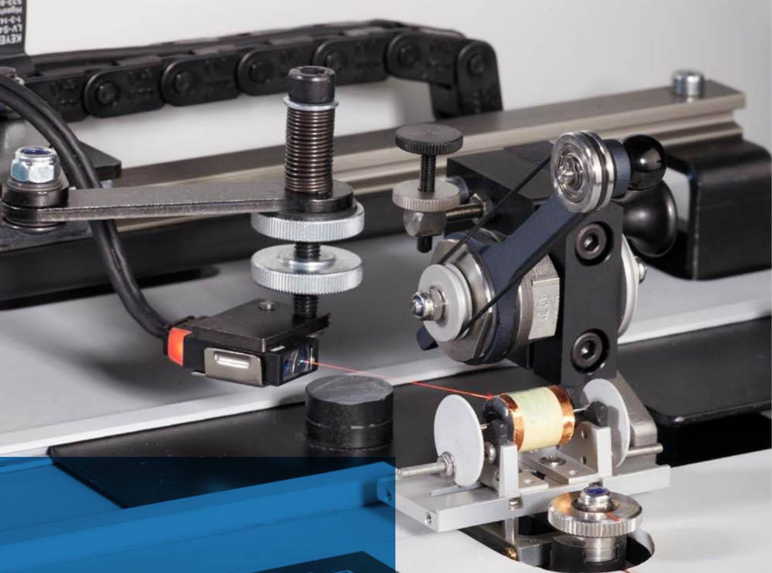
Easy setup of the laser scanning head for an even more accurate angle position (Pasio 005)
