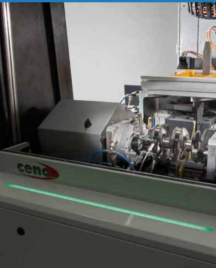
LED line provides clear information on the status of the machine and the crankshaft
